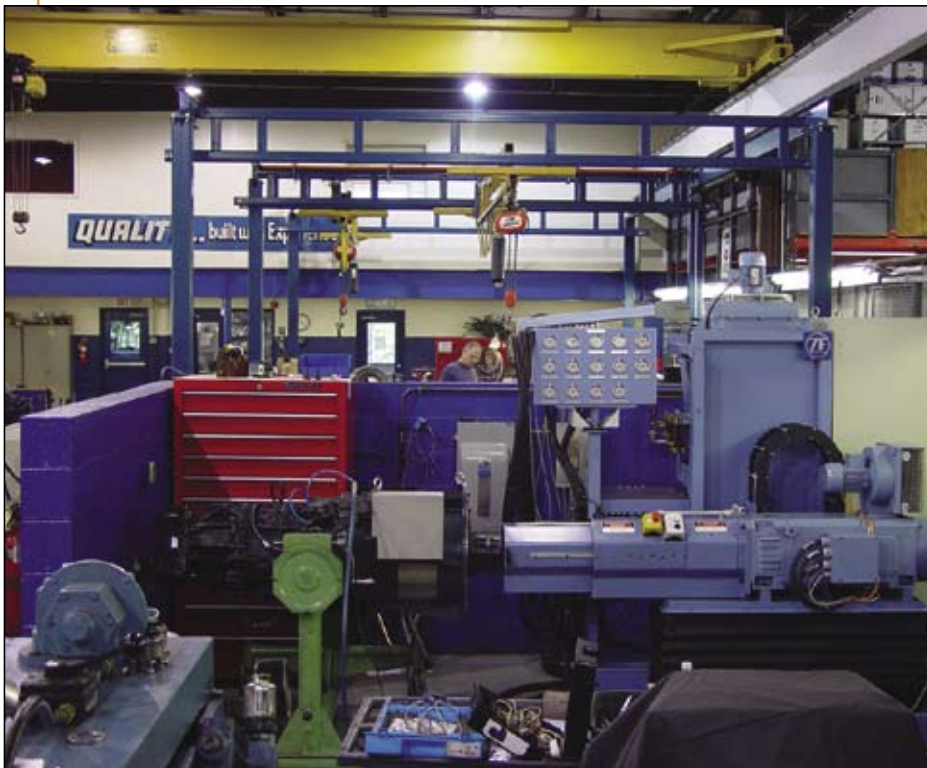
A rebuilt 12AS-2302 ZF AS-Tronic transmission from a Link-Belt crane undergoes standard testing procedures at the ZF factory.
