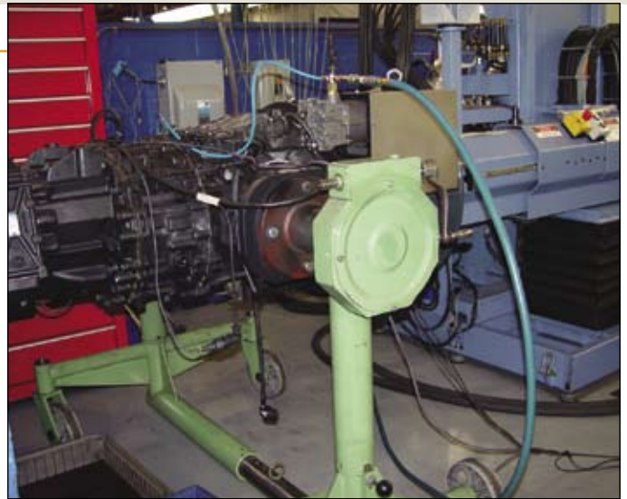
Left to right: The transmission output to the clutch and pressure plate along with air lines and diagnostic cables.
